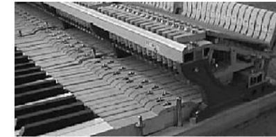
Fig G1- The bottom of a fully depressed key should barely clear the top of the rail guide for optimal performance.
