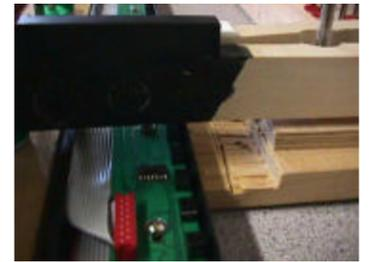
Fig C1- Place record strip on the key frame. Do not fasten it to the keyframe.
