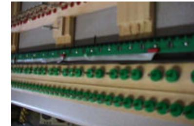
Fig H1- Fasten the rail frame to the keyframe by lifting the cables by the breaks and inserting screws.
